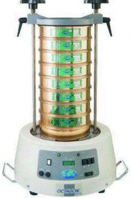
The high performance digital shaker For 200 mm & 8 in diameter sieves
